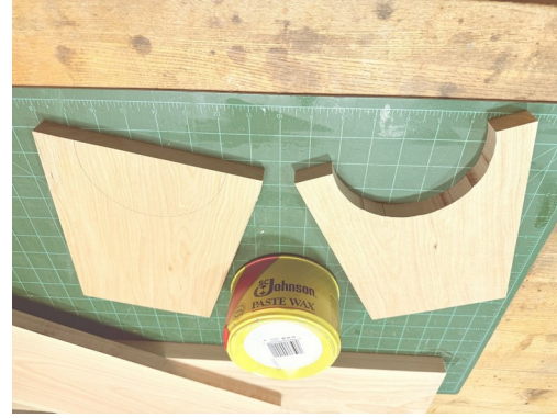
Both legs cut, with the waste from the relief cuts.
