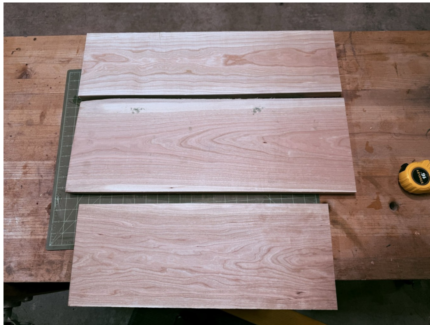
Stock milled to \frac{3}{4} " and crosscut to rough length, ready for ripping.
