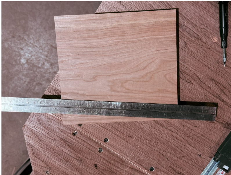
A leg blank ripped to width and squared up.
