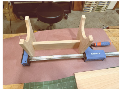
Clamped across the legs and stretcher.
