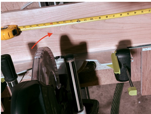
Leg clamped to the fence with the taper laid out.
