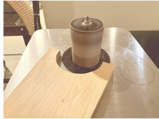
Fairing the arch to the line.
